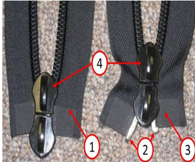
Fig. 1 Zipper Pin Misalignment
