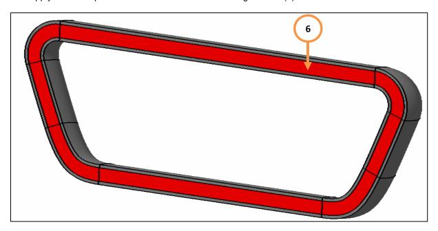
10. Remove the cover of the tape bonded into the monocoque and install the Service Disconnect seal onto the tape starting from the top left corner and moving clockwise as illustrated below (7).
