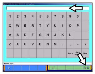
h. Click on the icon in the lower RH corner of the screen to have the MUT-III automatically read the VIN. If a message appears saying that the VIN cannot be input automatically, manually type the 17 digit VIN into the VIN field at the top of the page.
