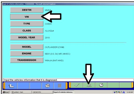
g. If the VIN or vehicle description displayed does not match the vehicle you are working on, click on the eraser icon at the bottom of the page to erase the existing data.
