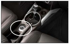
Mode selector button replaces rotary knob. Press the button to toggle through 2WD/4WD modes:
