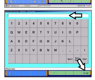
h. Click on the icon in the lower RH corner of the screen to have the MUT–III automatically read the VIN. If a message appears saying that the VIN cannot be input automatically, manually type the 17 digit VIN into the VIN field at the top of the page.
