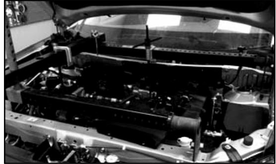
When using the engine support special tools as described, the front deck garnish (lower windshield trim) must be removed.
