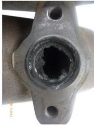
Figure 2 – Partially plugged AFI port
