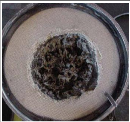
Media Damage from Over Fueling
