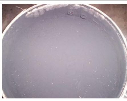
DPF face plugged – A face plugged DPF can be cleaned with OBFCT. Only use a cleaning machine if the engine does not start.
