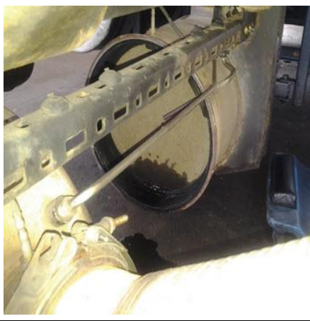
DPF Outlet Coolant - Oil Contaminated - Reusable
