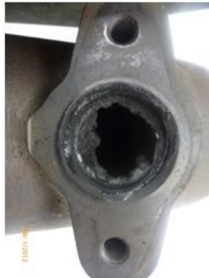
Figure 2 – Partially plugged AFI port
