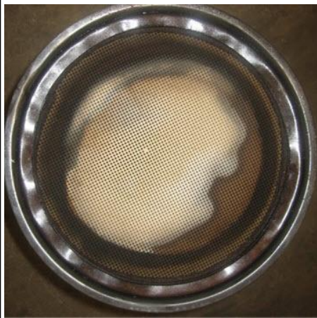
DPF Outlet - Oil Contaminated
