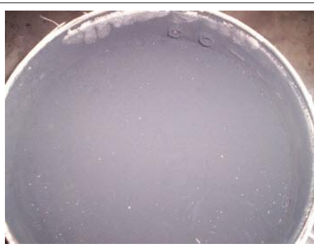
DPF face plugged – A face plugged DPF can be cleaned with OBFCT. Only use a cleaning machine if the engine does not start.
