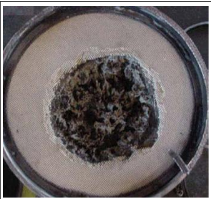
Media Damage from Over Fueling
