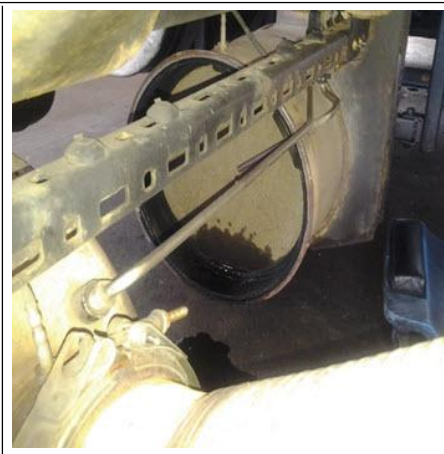
DPF Outlet Coolant - Oil Contaminated
