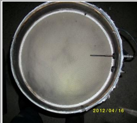
DPF Outlet Normal Operation
