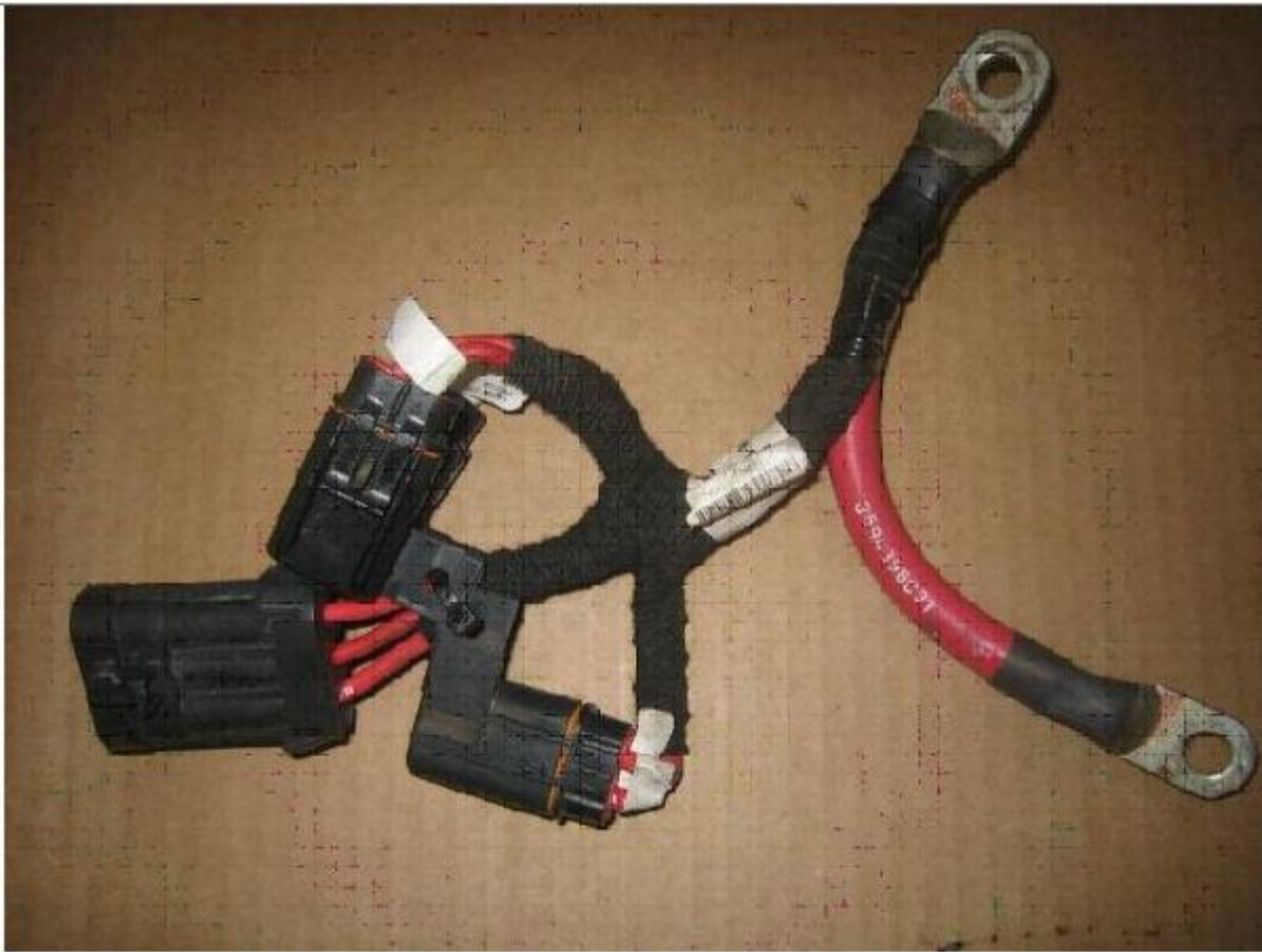
Figure 1. Jumper Cable Assembly - Typical
