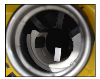
Insert the lockout mechanism into the filler neck and rotate from right-to-left <arrow> to seat properly into position.
