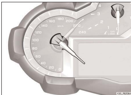
Example of Speedometer needle not in zero position
