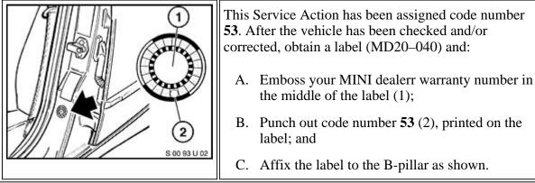
If the vehicle already has a label from a previous Service Action/Recall Campaign, affix the new label next to the old one. Do not affix one label on top of another one because a number from an underlying label could appear in the punched-out hole of the new label.
