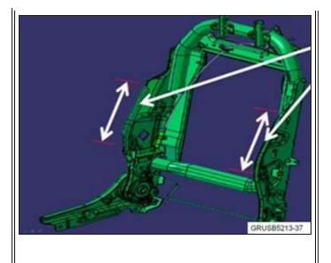
2. Refer to Repair Instruction 52 13 405 and remove the seat back padding, together with the seat cover, far enough to expose the surface corrosion on the metal seat back frame. The areas of concern are shown by the arrows.
