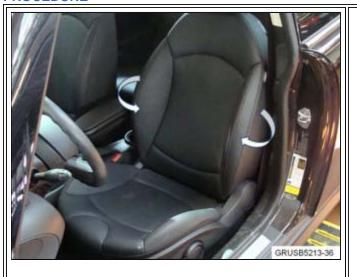
1. Duplicate the seat noise by moving the front seat back cover and padding left and then right. If the noise can be heard, proceed to the next step.
