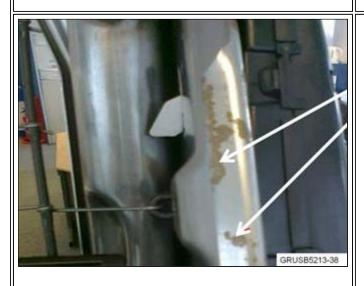
3. Remove the corrosion in two steps by first sanding with 320 grit sandpaper, and then finishing with 600 grit. Clean off the remaining dust from the seat back frame with a damp rag. When the surface is dry, uniformly apply a light coat of anti-friction agent Carbaflo KSP 105 to the sanded areas of the seat back frame. Reinstall the seat back padding and cover in the reverse order of its removal. Check the seat back again, and confirm the noise is gone.
