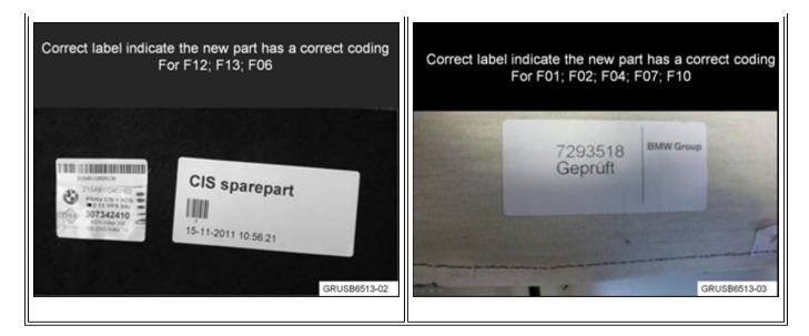
Install the replacement CIS mat in the vehicle and code the ACSM (Advanced Crash Safety Module) with ISTA/P.
