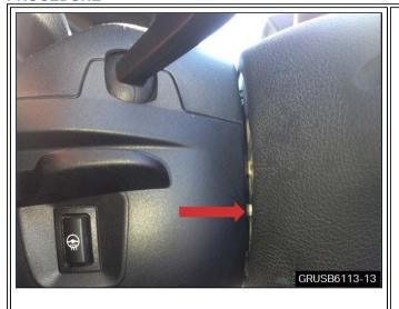
1. In the picture to the left, the white locking pin can be seen (from the driver's side) looking between the steering wheel and the column.
