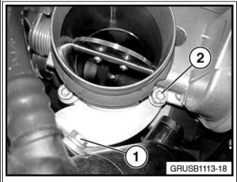
Reinstall the throttle valve and snug down all three throttle valve screws. Torque the two screws that are not attached to the new bracket to specification (8Nm). Tighten down the bracket bolt on the cylinder head (1) to 8Nm. Tighten the screw (2) holding the bracket to the throttle to 8 Nm.
