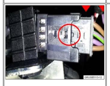
4. This close-up picture shows the 4-pin connector is slightly tilted and not fully inserted and locked in. The circle shows where the connector locking tab is located.
