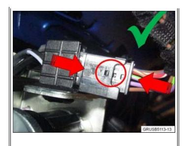
5. Push the connector in firmly until the locking tab is fully snapped into place. Check each electrical connector to make sure it is locked in by giving the wire harness a pull.
