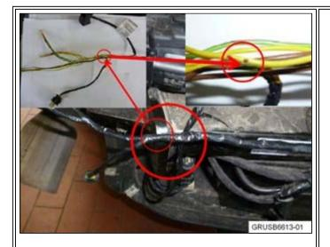
8. This picture shows a location where the rear PDC wire harness rubs against the trailer hitch if installed.
