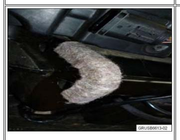
9. Apply felt strip to the trailer hitch in the location where the PDC wire harness rubs against the trailer hitch.
