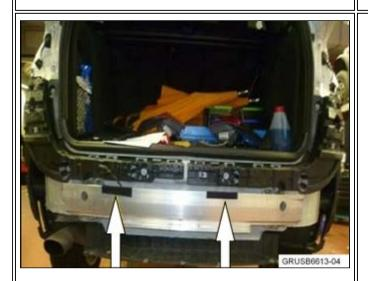
12. If needed, remove the rear bumper support. Refer to Repair Instruction RE5112050, "Removing and Installing Support for Rear Bumper Panel."
