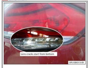
Condensation builds up inside the taillight lens.
