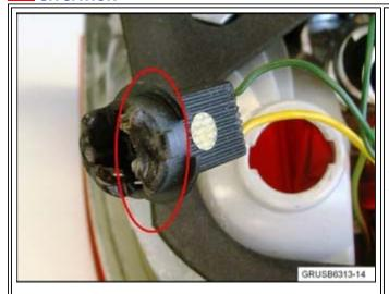
A Check Control message is displayed for brake light bulb failure. In some cases, inspection of the brake light bulb holder shows the molding for the bulb holder is deformed.
