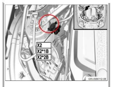
4. **X2 B+ Jump-starting point:**Check the metal brace located near the jump point terminal for signs of arcing. This can happen when jump-starting or the charging aid contacts the metal brace along with the terminal.
