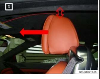
Photos C and D: The headrest and seatback must be able to move fore and aft without contacting the roof or sun visor, regardless of seat position. The headrest height will automatically adjust to maintain this clearance, regardless of seat position.
