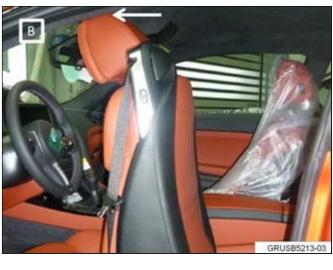
Photos A and B: In the event of an accident, the rear passenger must be able to move the front seatback forward, regardless of the seat position. This allows the rear passenger an easy exit from the rear seat of the vehicle, even if the electrical power source is no longer available.
