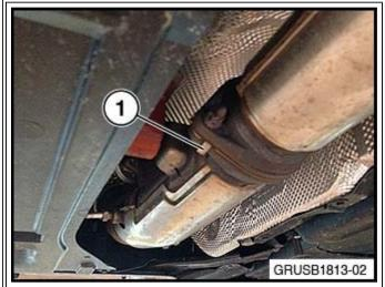
The barrel of the E70 mixer points toward the front of the car. This is easily identified by the mixer tabs wrapped around the front pipe flange (1).
