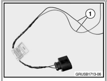
Cut the replacement harness (from connector repair kit P/N 61 11 9 312 324) at 50 mm away from the taped portion of the harness (1). Crimp the new level sensor harness to the body harness with the provided cable connectors and heat shrinking hose (Refer to Repair Instruction 61 13 ... Butt connector for repairing a plug connection). Install the new coolant expansion tank.
