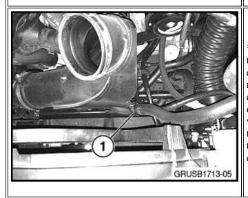
\*Note: Check for proper connection of the lower coolant hose from the expansion tank when removing/replacing the tank (1). The coolant hose may become disconnected during repairs. The hose will contact the engine cooling fan if this hose remains disconnected from the bracket. (Air box removed for clarity.)
