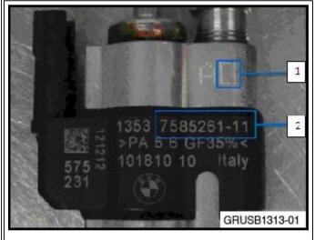
Additional Information: As of January 2013, an improved injector is available. Two distinct markings on the injector itself will identify the improved injector. 1 = Internal material improvement 2 = 7585261 – (index) 11 or greater
