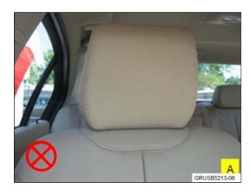
1. The headrest in picture A is lowered all the way down at the factory. This simplifies the seat installation and reduces damage on the production line. The headrest operation should be checked during PDI, and, once raised, the headrest will no longer lower down to the "installation" height. This is normal headrest operation and no repairs are needed. No new vehicle should be delivered to the customer with the front headrests in the "installation" position.
