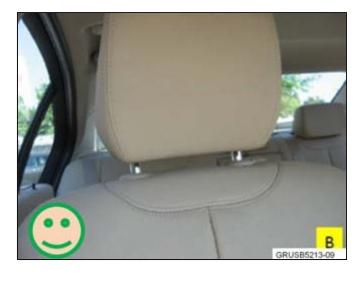
2. The headrest in picture B is in the correct lowered height position.
