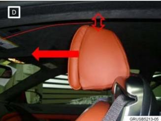
Photos C and D: The headrest and seatback must be able to move fore and aft without contacting the roof or sun visor, regardless of seat position. The headrest height will automatically adjust to maintain this clearance, regardless of seat position.
