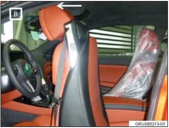
Photos A and B: In the event of an accident, the rear passenger must be able to move the front seatback forward, regardless of the seat position. This allows the rear passenger an easy exit from the rear seat of the vehicle, even if the electrical power source is no longer available.
