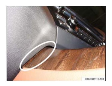
secured. Reinstall the center console trim, and check the effectiveness of the repair by pressing on the side trim again.
