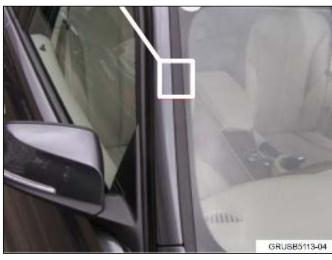
1. Confirm the noise is coming from the front windshield, near the left and/or right A-pillar area.
