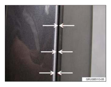
2. If a gap is seen between the affected A-pillar and the drip molding, the molding must be replaced. Refer to ISTA Repair Instruction 51 31 030, "Remove and install or replace the left or right side gutter strip." Install the replacement drip molding with the new blue colored clips listed below.
