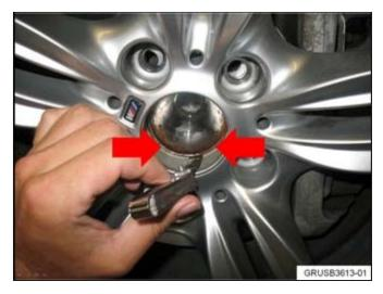
Check the wheel centering of the lightalloy rim on the wheel hub. To do so, clean the contact surfaces of the wheel hubs and the light-alloy rims, and only slightly tighten the wheels. Using a feeler gauge at the bottom position, determine the maximum play. Play of 0.1 mm is still within the permissible tolerance. Play of 0.15 mm or greater is outside the permissible tolerance.
