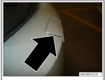
The customer may state the headlight nozzles are not flush with the front bumper, as shown. In this case, both left and right nozzle covers must be replaced.
