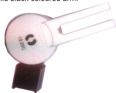
Latest level clutch potentiometer with solid white coloured arm
