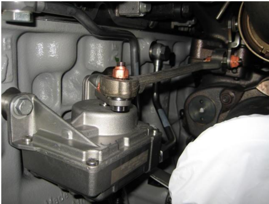
Figure 3 – DD13 System, Pull rod P/N Located On Top
