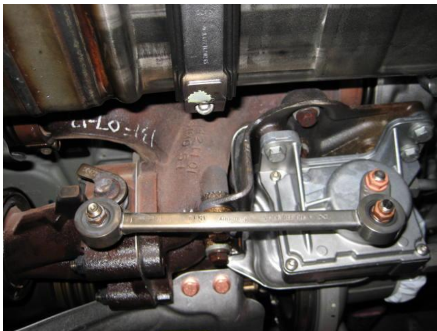
Figure 6 – DD15TC (472909) And DD16 System, Pull rod P/N Located On Top
