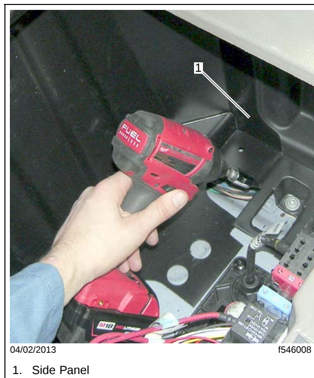
Fig. 2, Under Bunk Side Panel Removal
