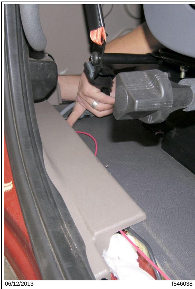
Fig. 9, Wire Fed into the Passenger-Side Harness Cover (daycabs)
