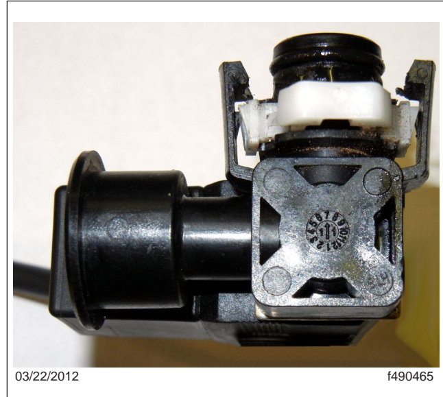
Fig. 2, 10-Watt Solenoid Valve ( 13.5\pm 0.7 \Omega )
