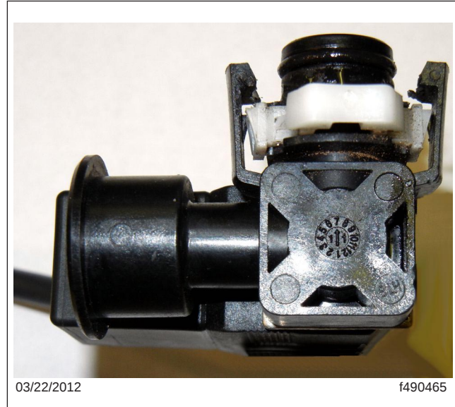
Fig. 2, 10-Watt Solenoid Valve (13.5±0.7 Ω)
