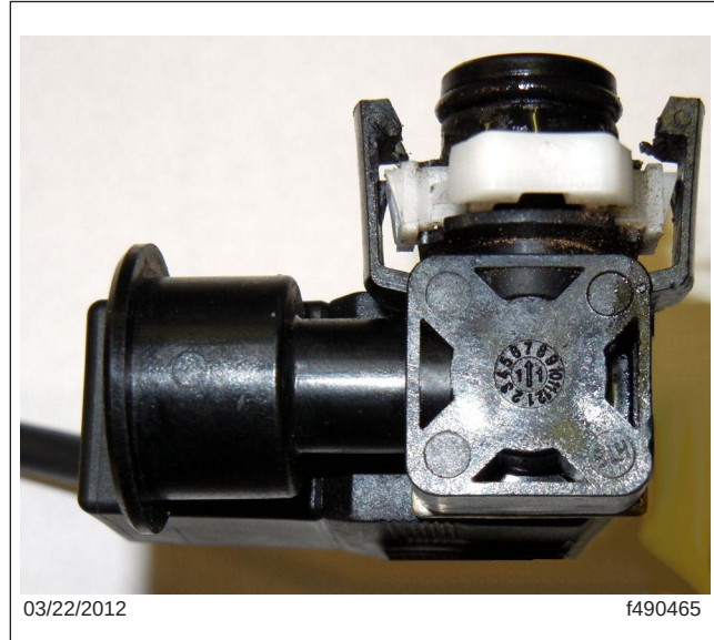
Fig. 2, 10-Watt Solenoid Valve ( 13.5\pm0.7\ \Omega )
