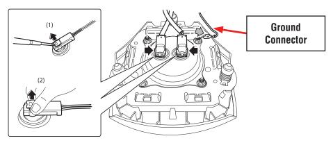
6. Disconnect the steering wheel wiring harness connector from the roll connector.
