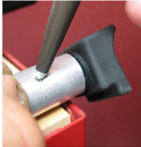
**Step 7-** Install the 2 pop rivets which position the tonneau cover material on the support pipe then touch up with a permanent black marker if necessary to complete the repair.
