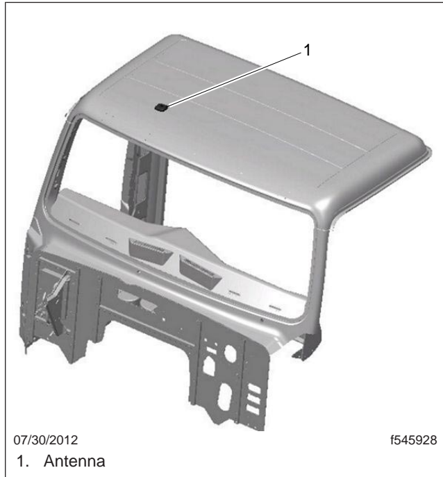
Fig. 8, Antenna Location, Daycab and Starlight Sleepercab
