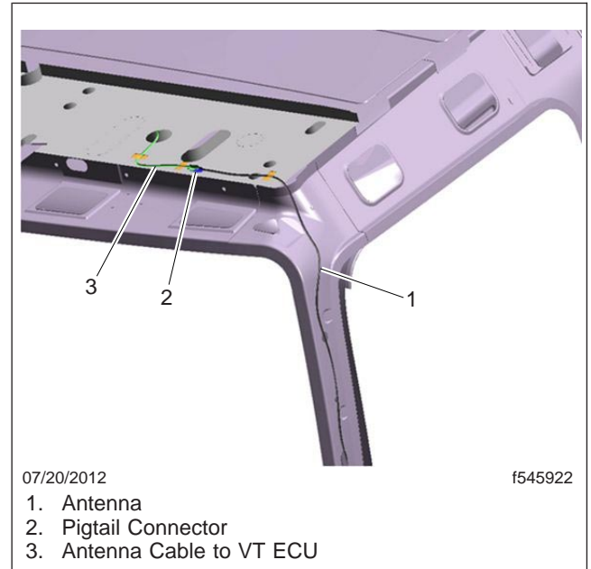
Fig. 9, Antenna Routing, Daycab and Starlight Sleepercab
