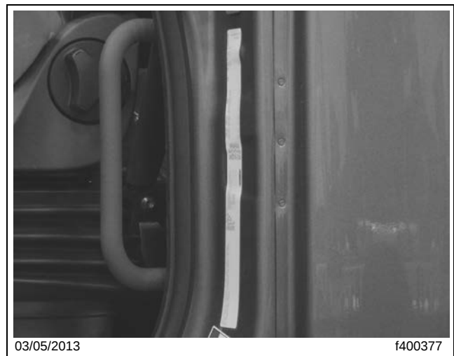
Fig. 4, The applied label should lie flat and with the same orientation as the existing label.
