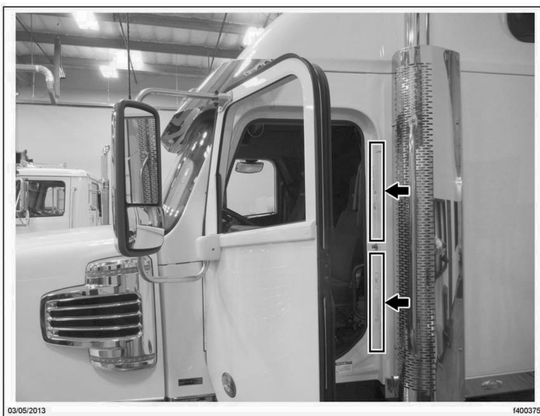
Fig. 1, The Vehicle Certification Door Label may be on the upper or lower portion of the driver's-side door frame.
