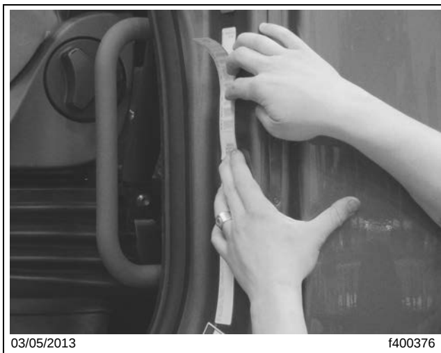
Fig. 3, Apply the label to the clean Vehicle Certification Door Label.
