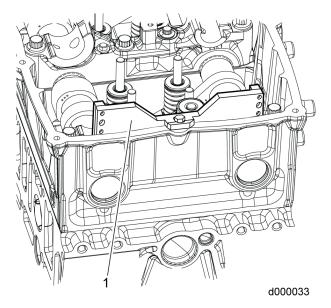
8. Verify that the marks on the gear teeth match the marks on the timing tool. If the marks do not match, research the root cause of incorrect camshaft timing.
