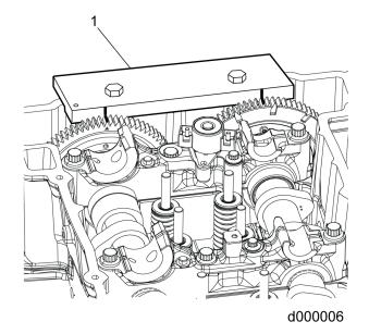
7. Install the front camshaft timing tool (1) into the grooves cut into the cams and hold it onto the camshaft housing with a bolt.
