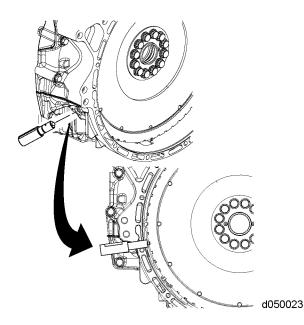
6. Install the rear camshaft timing tool (1) onto the camshaft housing.
