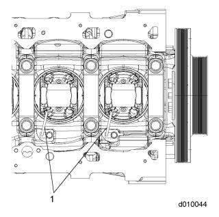
9. Position the crankshaft for each piston and connecting rod assembly to be removed at bottom dead center.
