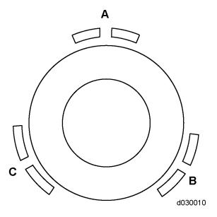
2. Allowable new ring end gaps for (A), (B), and (C) are shown below.
