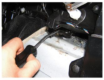
6. Push the carpet down with one hand, and with the other hand, take a pick tool and insert the tool in the grommet.
