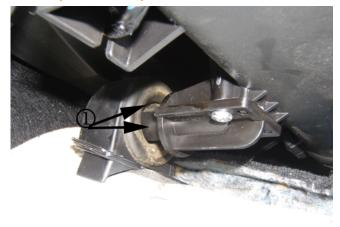
This condition may be caused by a collapsed A/C drain grommet (1), resulting in a wet carpet condition.
