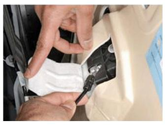
1. Disengage the door trim, without detaching the inside door handle cable. DO NOT LET THE TRIM PAD HANG FROM THE HANDLE CABLE OR THE WIRE HARNESS.
