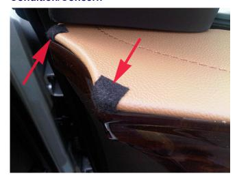
Two pieces of adhesive backed flocking material (black felt) are installed on the front side door interior trim panels as shown. This material is installed to protect the door panels during the build process.
